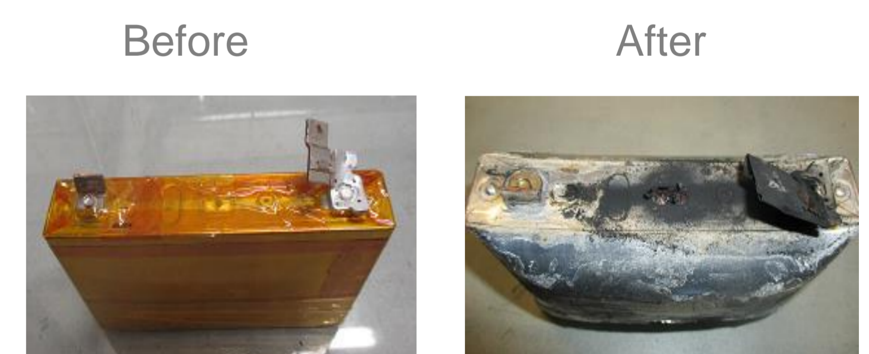
- Swelling of the cell. - Fire flame. - Ejection of material
